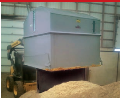
Sawdust Hoppers - 3/4 yd to 10 yd. capacity. Hooks up to your cyclone. Dump from operator seat.
