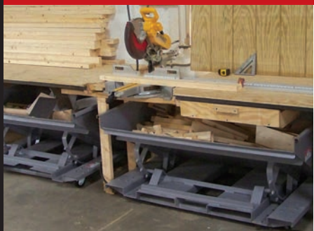
Baby Bull Hoppers with Bat-Wing bases. For restricted height areas
